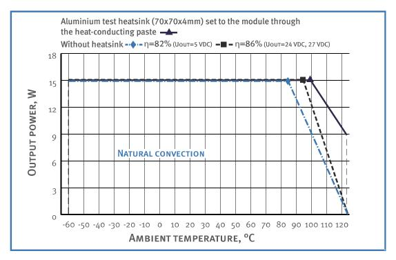
Dropping parts of the dashed and dash-dotted curves are in accordance with the **maximum temperature of the case**. Output power must not exceed the values which are limited by corresponding curve for a given ambient temperature.
